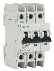
Eaton miniature circuit breaker, current-limiting, 2A, 480Y / 277 VAC / 96 VDC, 3-pole, C curve, thermal magnetic, 10kA @ 480Y/277 VAC interrupting rating, 35mm DIN rail mount.
