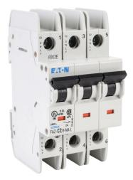
Eaton miniature circuit breaker, current-limiting, 2A, 240 VAC / 96 VDC, 3-pole, C curve, thermal magnetic, 10kA @ 240 VAC interrupting rating, 35mm DIN rail mount.
