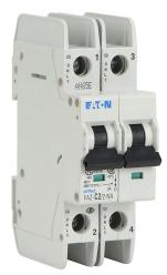
Eaton miniature circuit breaker, current-limiting, 2A, 480Y / 277 VAC / 96 VDC, 2-pole, C curve, thermal magnetic, 10kA @ 480Y/277 VAC interrupting rating, 35mm DIN rail mount.
