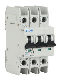
Eaton miniature circuit breaker, current-limiting, 1.5A, 480Y / 277 VAC / 96 VDC, 3-pole, C curve, thermal magnetic, 10kA @ 480Y/277 VAC interrupting rating, 35mm DIN rail mount.
