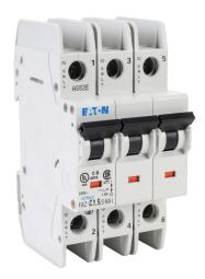
Eaton miniature circuit breaker, current-limiting, 1.5A, 240 VAC / 96 VDC, 3-pole, C curve, thermal magnetic, 10kA @ 240 VAC interrupting rating, 35mm DIN rail mount.
