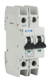
Eaton miniature circuit breaker, current-limiting, 1.5A, 480Y / 277 VAC / 96 VDC, 2-pole, C curve, thermal magnetic, 10kA @ 480Y/277 VAC interrupting rating, 35mm DIN rail mount.
