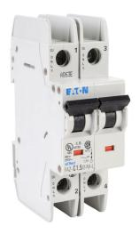
Eaton miniature circuit breaker, current-limiting, 1.5A, 240 VAC / 96 VDC, 2-pole, C curve, thermal magnetic, 10kA @ 240 VAC interrupting rating, 35mm DIN rail mount.
