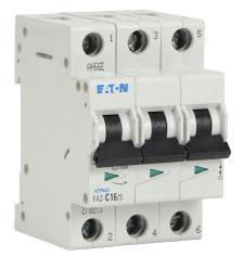
Eaton miniature supplementary protector, 16A, 480Y / 277 VAC / 96 VDC, 3-pole, C curve, thermal magnetic, 10kA @ 480Y/277 VAC interrupting rating, 35mm DIN rail mount.
