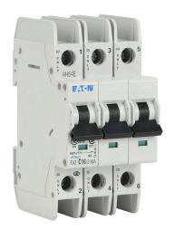
Eaton miniature circuit breaker, current-limiting, 16A, 480Y / 277 VAC / 96 VDC, 3-pole, C curve, thermal magnetic, 14kA @ 480Y/277 VAC interrupting rating, 35mm DIN rail mount.
