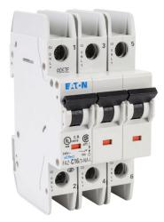
Eaton miniature circuit breaker, current-limiting, 16A, 240 VAC / 96 VDC, 3-pole, C curve, thermal magnetic, 14kA @ 240 VAC interrupting rating, 35mm DIN rail mount.
