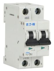
Eaton miniature supplementary protector, 16A, 480Y / 277 VAC / 96 VDC, 2-pole, C curve, thermal magnetic, 10kA @ 480Y/277 VAC interrupting rating, 35mm DIN rail mount.
