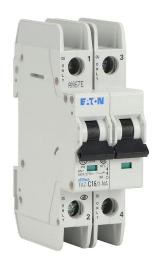
Eaton miniature circuit breaker, current-limiting, 16A, 480Y / 277 VAC / 96 VDC, 2-pole, C curve, thermal magnetic, 14kA @ 480Y/277 VAC interrupting rating, 35mm DIN rail mount.
