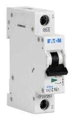
Eaton miniature supplementary protector, 16A, 277 VAC / 48 VDC, 1-pole, C curve, thermal magnetic, 10kA @ 277 VAC interrupting rating, 35mm DIN rail mount.
