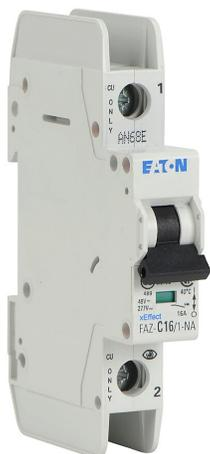
Eaton miniature circuit breaker, current-limiting, 16A, 277 VAC / 48 VDC, 1-pole, C curve, thermal magnetic, 14kA @ 277 VAC interrupting rating, 35mm DIN rail mount.
