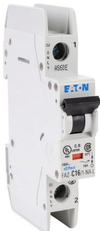
Eaton miniature circuit breaker, current-limiting, 16A, 240 VAC / 48 VDC, 1-pole, C curve, thermal magnetic, 14kA @ 240 VAC interrupting rating, 35mm DIN rail mount.
