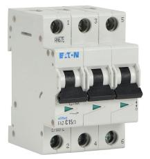
Eaton miniature supplementary protector, 15A, 480Y / 277 VAC / 96 VDC, 3-pole, C curve, thermal magnetic, 10kA @ 480Y/277 VAC interrupting rating, 35mm DIN rail mount.
