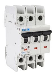
Eaton miniature circuit breaker, current-limiting, 15A, 240 VAC / 96 VDC, 3-pole, C curve, thermal magnetic, 14kA @ 240 VAC interrupting rating, 35mm DIN rail mount.
