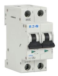
Eaton miniature supplementary protector, 15A, 480Y / 277 VAC / 96 VDC, 2-pole, C curve, thermal magnetic, 10kA @ 480Y/277 VAC interrupting rating, 35mm DIN rail mount.
