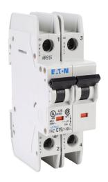
Eaton miniature circuit breaker, current-limiting, 15A, 240 VAC / 96 VDC, 2-pole, C curve, thermal magnetic, 14kA @ 240 VAC interrupting rating, 35mm DIN rail mount.
