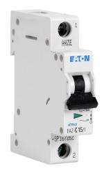
Eaton miniature supplementary protector, 15A, 277 VAC / 48 VDC, 1-pole, C curve, thermal magnetic, 10kA @ 277 VAC interrupting rating, 35mm DIN rail mount.
