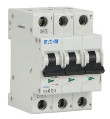
Eaton miniature supplementary protector, 13A, 480Y / 277 VAC / 96 VDC, 3-pole, C curve, thermal magnetic, 10kA @ 480Y/277 VAC interrupting rating, 35mm DIN rail mount.
