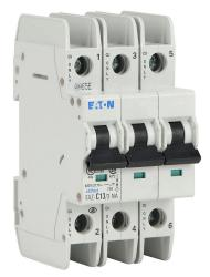
Eaton miniature circuit breaker, current-limiting, 13A, 480Y / 277 VAC / 96 VDC, 3-pole, C curve, thermal magnetic, 10kA @ 480Y/277 VAC interrupting rating, 35mm DIN rail mount.
