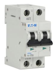
Eaton miniature supplementary protector, 13A, 480Y / 277 VAC / 96 VDC, 2-pole, C curve, thermal magnetic, 10kA @ 480Y/277 VAC interrupting rating, 35mm DIN rail mount.
