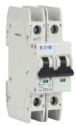
Eaton miniature circuit breaker, current-limiting, 13A, 480Y / 277 VAC / 96 VDC, 2-pole, C curve, thermal magnetic, 10kA @ 480Y/277 VAC interrupting rating, 35mm DIN rail mount.
