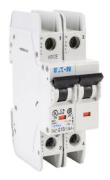
Eaton miniature circuit breaker, current-limiting, 13A, 240 VAC / 96 VDC, 2-pole, C curve, thermal magnetic, 10kA @ 240 VAC interrupting rating, 35mm DIN rail mount.
