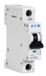
Eaton miniature supplementary protector, 13A, 277 VAC / 48 VDC, 1-pole, C curve, thermal magnetic, 10kA @ 277 VAC interrupting rating, 35mm DIN rail mount.
