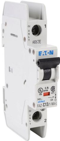
Eaton miniature circuit breaker, current-limiting, 13A, 240 VAC / 48 VDC, 1-pole, C curve, thermal magnetic, 10kA @ 240 VAC interrupting rating, 35mm DIN rail mount.
