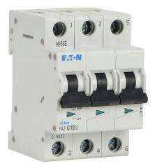
Eaton miniature supplementary protector, 10A, 480Y / 277 VAC / 96 VDC, 3-pole, C curve, thermal magnetic, 10kA @ 480Y/277 VAC interrupting rating, 35mm DIN rail mount.
