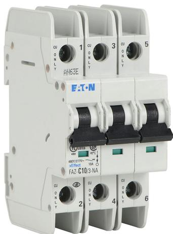
Eaton miniature circuit breaker, current-limiting, 10A, 480Y / 277 VAC / 96 VDC, 3-pole, C curve, thermal magnetic, 10kA @ 480Y/277 VAC interrupting rating, 35mm DIN rail mount.
