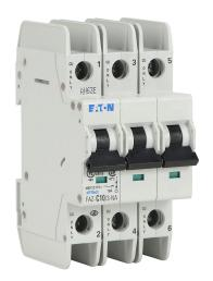
Eaton miniature circuit breaker, current-limiting, 10A, 480Y / 277 VAC / 96 VDC, 3-pole, C curve, thermal magnetic, 10kA @ 480Y/277 VAC interrupting rating, 35mm DIN rail mount.
