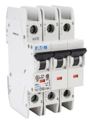
Eaton miniature circuit breaker, current-limiting, 10A, 240 VAC / 96 VDC, 3-pole, C curve, thermal magnetic, 10kA @ 240 VAC interrupting rating, 35mm DIN rail mount.
