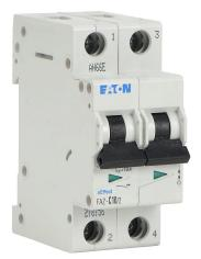
Eaton miniature supplementary protector, 10A, 480Y / 277 VAC / 96 VDC, 2-pole, C curve, thermal magnetic, 10kA @ 480Y/277 VAC interrupting rating, 35mm DIN rail mount.
