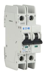
Eaton miniature circuit breaker, current-limiting, 10A, 480Y / 277 VAC / 96 VDC, 2-pole, C curve, thermal magnetic, 10kA @ 480Y/277 VAC interrupting rating, 35mm DIN rail mount.
