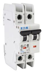
Eaton miniature circuit breaker, current-limiting, 10A, 240 VAC / 96 VDC, 2-pole, C curve, thermal magnetic, 10kA @ 240 VAC interrupting rating, 35mm DIN rail mount.
