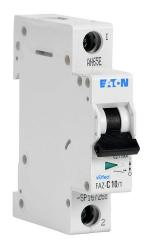
Eaton miniature supplementary protector, 10A, 277 VAC / 48 VDC, 1-pole, C curve, thermal magnetic, 10kA @ 277 VAC interrupting rating, 35mm DIN rail mount.
