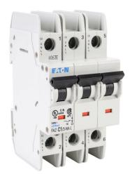
Eaton miniature circuit breaker, current-limiting, 1A, 240 VAC / 96 VDC, 3-pole, C curve, thermal magnetic, 10kA @ 240 VAC interrupting rating, 35mm DIN rail mount.
