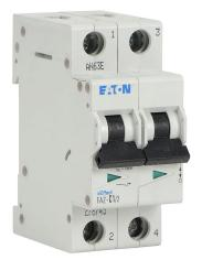
Eaton miniature supplementary protector, 1A, 480Y / 277 VAC / 96 VDC, 2-pole, C curve, thermal magnetic, 10kA @ 480Y/277 VAC interrupting rating, 35mm DIN rail mount.
