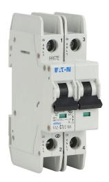
Eaton miniature circuit breaker, current-limiting, 1A, 480Y / 277 VAC / 96 VDC, 2-pole, C curve, thermal magnetic, 10kA @ 480Y/277 VAC interrupting rating, 35mm DIN rail mount.
