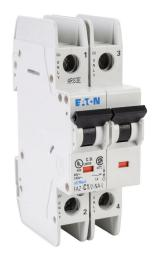
Eaton miniature circuit breaker, current-limiting, 1A, 240 VAC / 96 VDC, 2-pole, C curve, thermal magnetic, 10kA @ 240 VAC interrupting rating, 35mm DIN rail mount.
