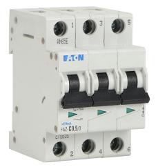
Eaton miniature supplementary protector, 0.5A, 480Y / 277 VAC / 96 VDC, 3-pole, C curve, thermal magnetic, 10kA @ 480Y/277 VAC interrupting rating, 35mm DIN rail mount.
