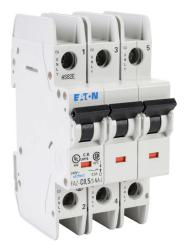
Eaton miniature circuit breaker, current-limiting, 0.5A, 240 VAC / 96 VDC, 3-pole, C curve, thermal magnetic, 10kA @ 240 VAC interrupting rating, 35mm DIN rail mount.
