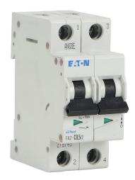
Eaton miniature supplementary protector, 0.5A, 480Y / 277 VAC / 96 VDC, 2-pole, C curve, thermal magnetic, 10kA @ 480Y/277 VAC interrupting rating, 35mm DIN rail mount.
