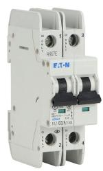
Eaton miniature circuit breaker, current-limiting, 0.5A, 480Y / 277 VAC / 96 VDC, 2-pole, C curve, thermal magnetic, 10kA @ 480Y/277 VAC interrupting rating, 35mm DIN rail mount.
