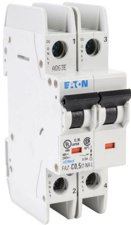
Eaton miniature circuit breaker, current-limiting, 0.5A, 240 VAC / 96 VDC, 2-pole, C curve, thermal magnetic, 10kA @ 240 VAC interrupting rating, 35mm DIN rail mount.
