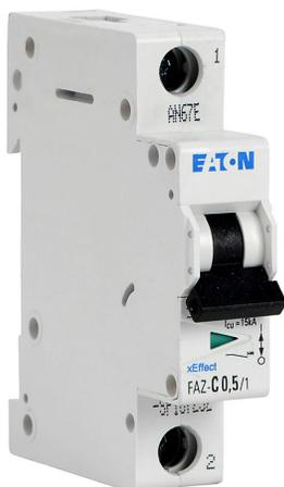
Eaton miniature supplementary protector, 0.5A, 277 VAC / 48 VDC, 1-pole, C curve, thermal magnetic, 10kA @ 277 VAC interrupting rating, 35mm DIN rail mount.
