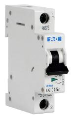
Eaton miniature supplementary protector, 0.5A, 277 VAC / 48 VDC, 1-pole, C curve, thermal magnetic, 10kA @ 277 VAC interrupting rating, 35mm DIN rail mount.
