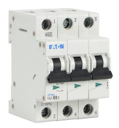
Eaton miniature supplementary protector, 8A, 480Y / 277 VAC / 96 VDC, 3-pole, B curve, thermal magnetic, 10kA @ 480Y/277 VAC interrupting rating, 35mm DIN rail mount.
