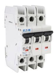
Eaton miniature circuit breaker, current-limiting, 8A, 480Y / 277 VAC / 96 VDC, 3-pole, B curve, thermal magnetic, 10kA @ 480Y/277 VAC interrupting rating, 35mm DIN rail mount.
