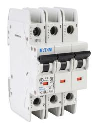
Eaton miniature circuit breaker, current-limiting, 8A, 240 VAC / 96 VDC, 3-pole, B curve, thermal magnetic, 10kA @ 240 VAC interrupting rating, 35mm DIN rail mount.
