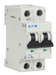
Eaton miniature supplementary protector, 8A, 480Y / 277 VAC / 96 VDC, 2-pole, B curve, thermal magnetic, 10kA @ 480Y/277 VAC interrupting rating, 35mm DIN rail mount.
