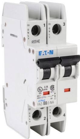
Eaton miniature circuit breaker, current-limiting, 8A, 480Y / 277 VAC / 96 VDC, 2-pole, B curve, thermal magnetic, 10kA @ 480Y/277 VAC interrupting rating, 35mm DIN rail mount.
