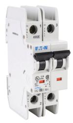
Eaton miniature circuit breaker, current-limiting, 8A, 240 VAC / 96 VDC, 2-pole, B curve, thermal magnetic, 10kA @ 240 VAC interrupting rating, 35mm DIN rail mount.
