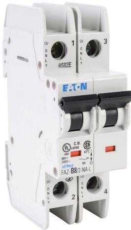
Eaton miniature circuit breaker, current-limiting, 8A, 240 VAC / 96 VDC, 2-pole, B curve, thermal magnetic, 10kA @ 240 VAC interrupting rating, 35mm DIN rail mount.
